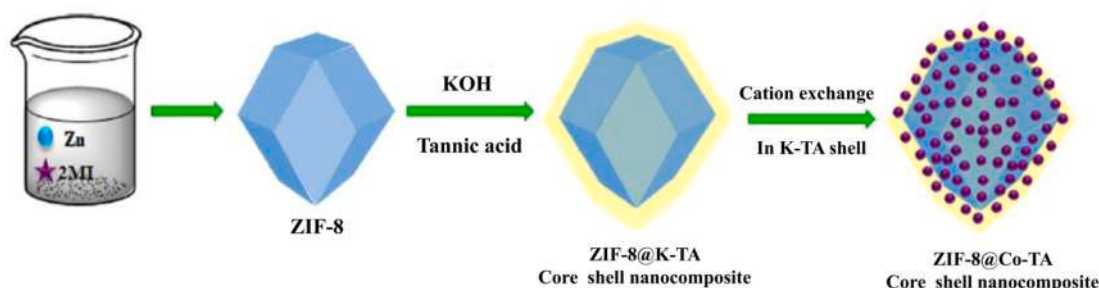
Fig. 12. Possible growth mechanism of ZIF-8@Co-TA nanocomposite. [Reprinted with permission from ref [85]. Copyright 2020, Elsevier.]
